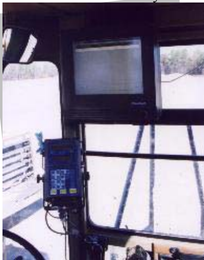
Cab Mounted Loadout Terminal
